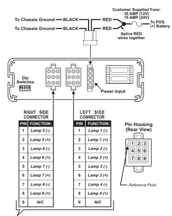
NOTE: These are the functions of the PIN connectors on the back of the control head. Refer to your Traffic Advisor manual for your specific input cable wire functions.
