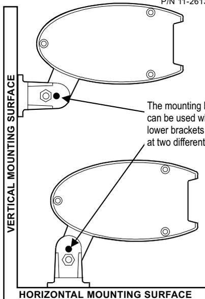
The mounting brackets have two holes that can be used while attaching the upper and lower brackets together, to position the T/A at two different heights.
