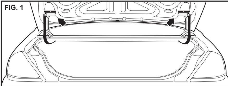
This bracket will mount to the inside of the trunk using one of the two bolts that hold the trunk hinges on.
