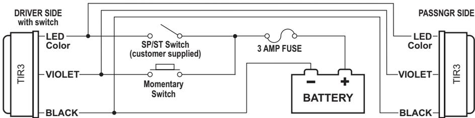
**Low Power:** To activate low power, press the momentary switch for less than 1 second. This will set the lighthead into low power. To switch the lighthead back to high power\*, turn the unit off and then back on.
