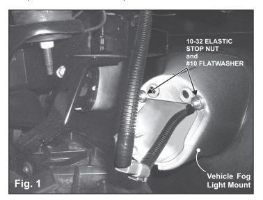
2. Unplug the existing fog light from the wiring harness, remove mounting hardware and remove the fog light from the vehicle. If the vehicle is not equipped with fog lights remove the
