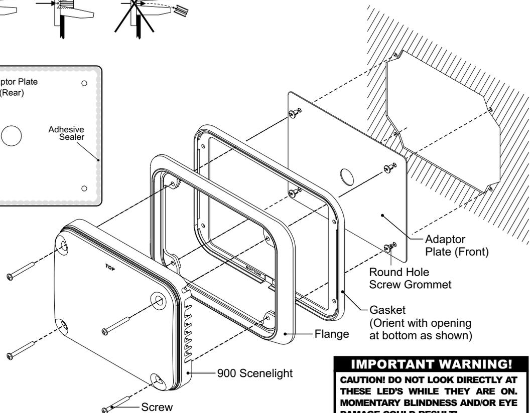
4. Route the wires through the flange (if present) and gasket. Extend the wires through the wire passage hole, make the appropriate connections and confirm proper operation of the light (refer to the guide included with your lighthouse for important wiring and fusing information).
