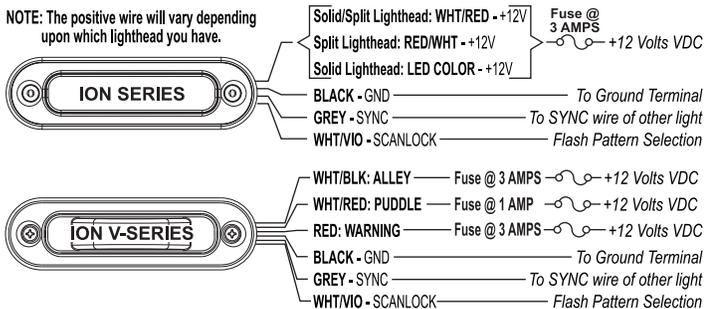
**WARNING: All customer supplied wires that connect to the positive terminal of the battery must be sized to supply at least 125% of the maximum operating current and FUSED at the battery to carry that load. DO NOT USE CIRCUIT BREAKERS WITH THIS PRODUCT!**
