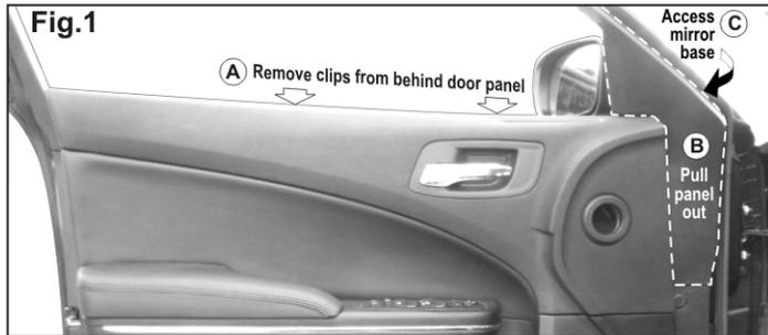
2. Carefully pull the panel covering mirror base away and remove the three nuts holding the mirror assembly on, unplug the wiring and remove the mirror assembly from the vehicle.
