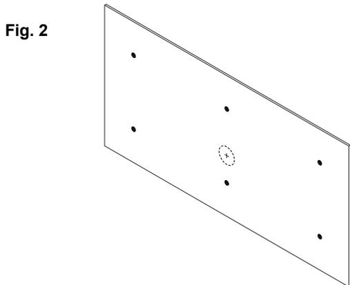
4. Drill the mounting holes at the areas indicated using an appropriately sized drill bit. Create the wire passage hole using an appropriately sized hole saw. Be sure to de-burr each hole before continuing.
