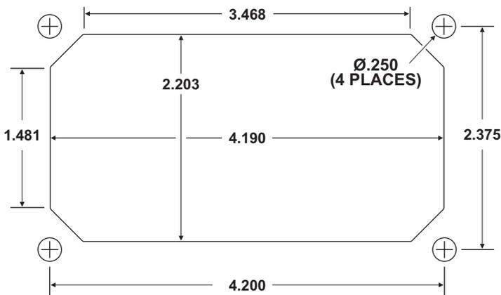
**NOTE: HORIZONTAL MOUNTING PATTERN IS SHOWN. PATTERN WOULD BE ROTATED 90° FOR VERTICAL MOUNTING.**
