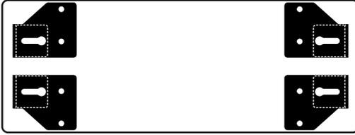
here. When positioned as shown, the mounting holes from the new lightbar will match the footprint of the lightbar you are replacing. Adjust as necessary so the lightbar sits properly on the vehicle and add spacers if necessary (See below). Make sure mounting hardware is tightened to 14 In. Lbs.
