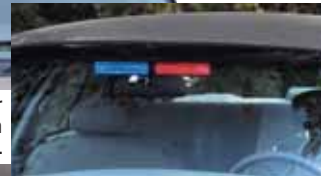
Dual SlimLighters mounted to headliner in rear hatch of vehicle.
