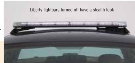
NEW! 44" Justice lightbar mounting foot shown on a 2008 Ford Crown Vic (see dimension drawing)
