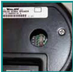
(Water resistant rubber plug shown removed to show mode switches and fuse).
