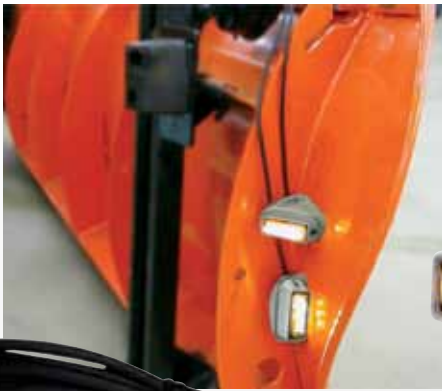
WFLOW3A Two light system for complete protection when plow is in operation or stowed
