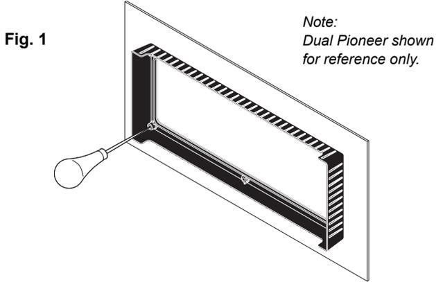
2. Using an awl or similar tool, mark the areas where the mounting holes are to be drilled. After the mounting holes have been scribed, remove the cover and confirm that the areas marked precisely match the appropriate mounting dimensions shown on page 3.
