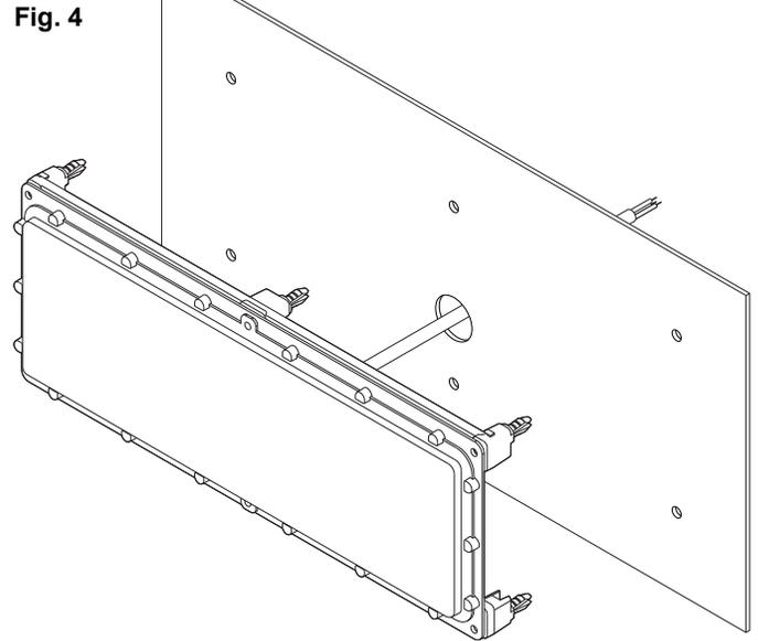
7. With the assembly pressed firmly against the mounting surface, place the Pioneer cover onto the assembly (Fig.5). Insert the mounting screws provided through the cover and into the mounting clips. Using a torque wrench, tighten the mounting screws until a value of 15-18 in/lbs is achieved.
