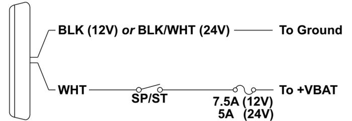
**Waterproof butt splices and/or connectors are required if that connection could be exposed to moisture. Any unused wires must be sealed (waterproofed) to prevent moisture infiltration.**
