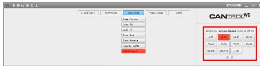
On the **CANport** tab we can select the signal and the **Press/State** we want to program. Depending on the Signal selected you will have multiple **Presses/States**
