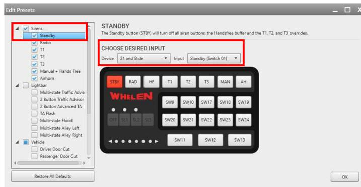
To setup Presets we first select one by checking it, then we select where it will be programmed. In this example, selecting Standby, and placing it on Control Head Switch 01
