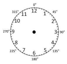
Flashing starts at Phase one 0° degrees. Phase one 0° degrees and phase two 180° degrees alternate with each other. Setting eight modules from 0°degrees to 315°degrees on our clock would allow our flash pattern to rotate clockwise.
