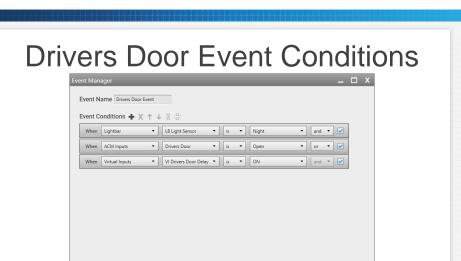
Set the three Event Conditions so the Drivers Door Cut and Delay only work at night
