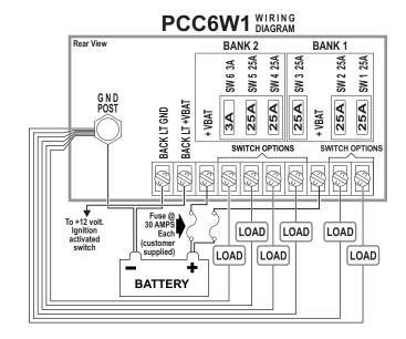
**BCKLT +V:** This terminal supplies power to the units window backlighting. This terminal can be connected to any ignition controlled +VBAT power source that can supply 100ma.
