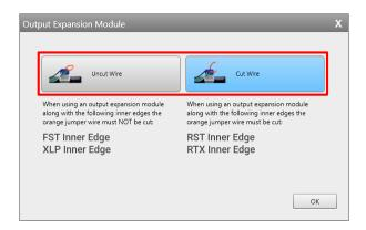
To ensure the proper operation of the **Output Expansion** module, pay attention to the orange wire being **Cut** or **Uncut**
