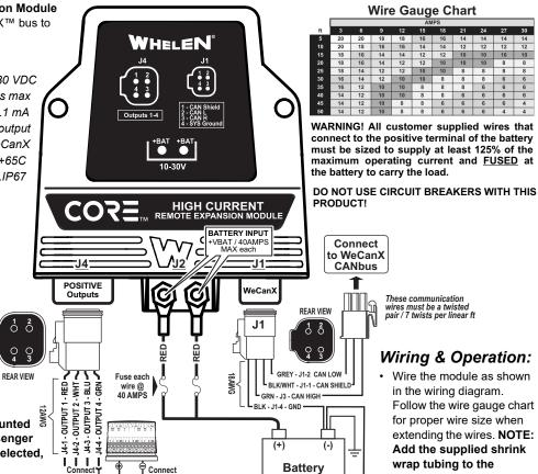
Extend the WeCanX wires to the CenCom Core™ Main Box and connect them as shown. Operation is controlled by CenCom Core™.
