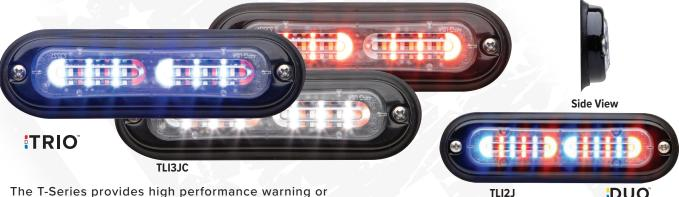
The T-Series provides high performance warning or illumination and features a sleek and low-profile design, with a depth of only 0.5".
